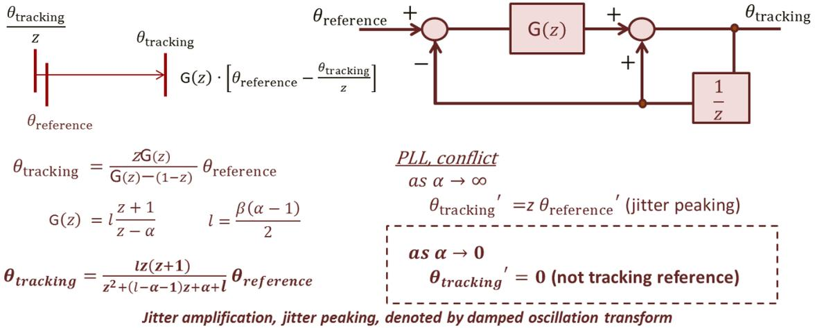
"It has been widely known that the traditional PLL inherently has jitter peaking that cannot be eliminated."
