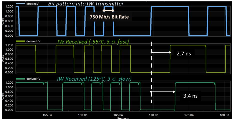
Figure 3. High bitrates with negligible latencies, transmitter to adjacent receiver with 60 dBm power at receiver.
