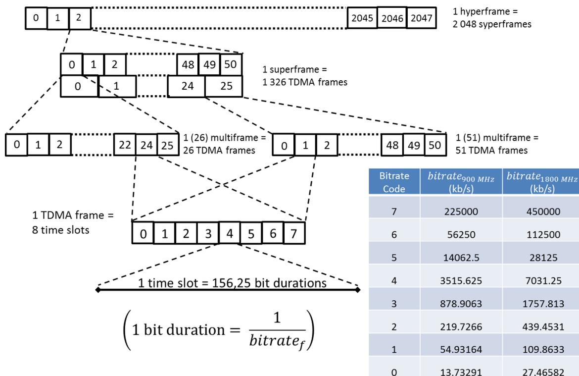
Figure 7. IW GSM physical layer, minimal impact to existing specification.
