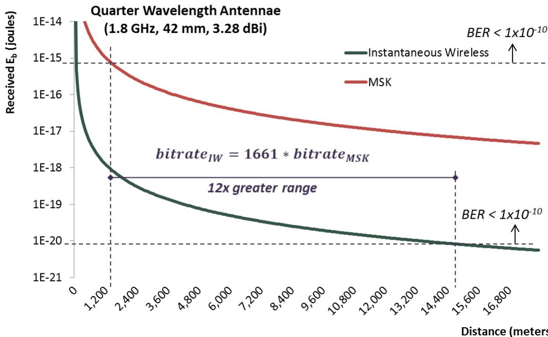
Figure 5. IW, at 1661x higher bitrate, transmits 12x further when both IW and MSK are set to the same reliability.
