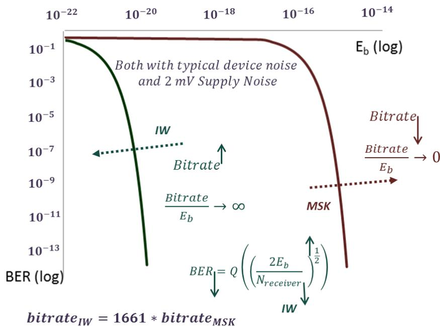
Figure 4. IW reduces BER with high bitrate, eliminating the bitrate to reliability tradeoff of quadrature modulations.
